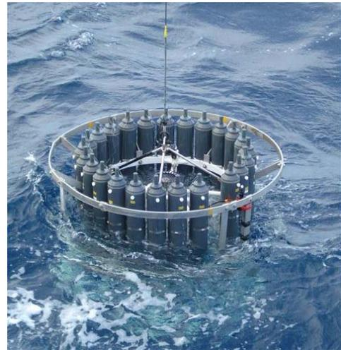
A CTD (Conductivity, Temperature, Depth) rosette is deployed. Photo by Lance A. Fujieki
