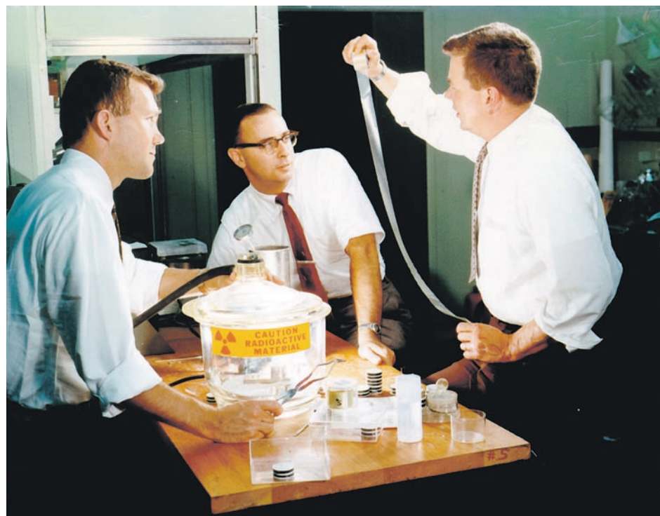
Figure 2. "PIE"-oneers P.B. Price (left), R. L. Fleischer (center) and R. M. Walker (right) at their laboratory at GERL circa 1963. Walker is holding a Lexan ® strip that had been irradiated by 252 Cf fission fragments in the bell jar on the center of the table. From Fleischer (1998), courtesy of the author.
