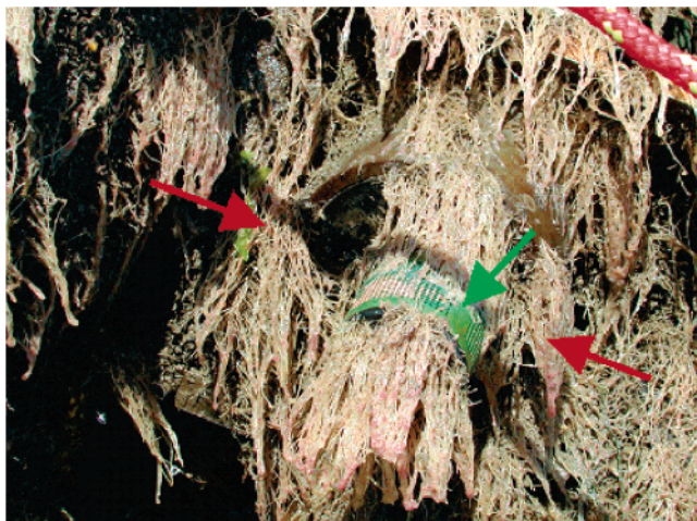
Figure 3. An ISUS optical nitrate sensor encrusted with hydroids. Red arrows identify the outside diameter of the instrument (12.5 cm), and the green arrow points to a copper antifouling shield that protects the optics. Used with permission. Copyright 2006, MBARI.
