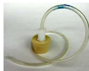
1 piece of rubber tubing connected with a straight connector at one end to a large, white stopper
