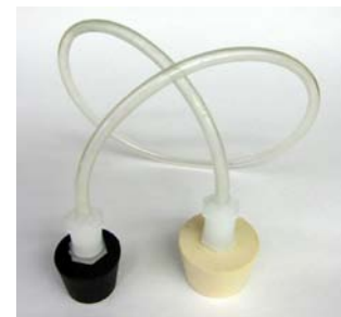
5 pieces of rubber tubing connected with straight connectors to a small, black stopper (#6) at one end and a large, white stopper at the other (#8)
