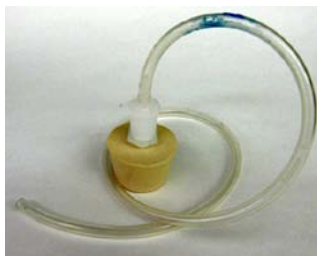
5 pieces of rubber tubing connected with a straight connector at one end to a large, white stopper (#8)
