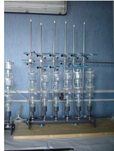
Size-fractionation filtration system used in the in vivo ETS method.
