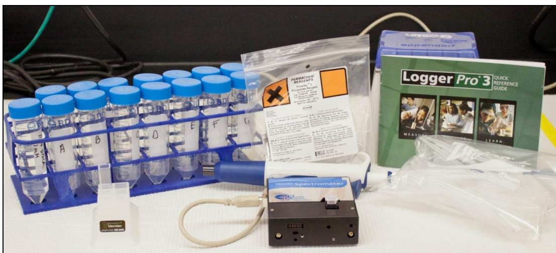
A subset of the components included in a single science kit: including a Vernier spectrophotometer, software, chemical reagents, pipettes and tubes for a standard curve.
