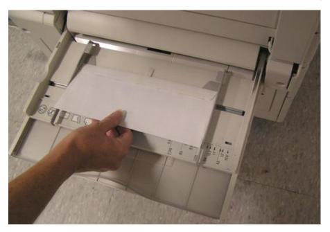
3. Center the stack of envelopes, then slide the paper edge guides until they are just touching the edges of the stack.
