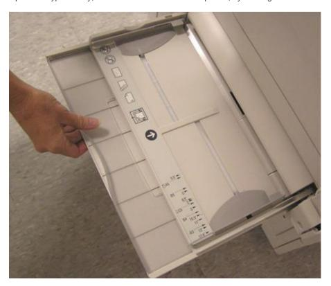
2. Load the envelopes in the tray with the flaps closed, flaps up, and flaps on the leading edge (toward the right).
