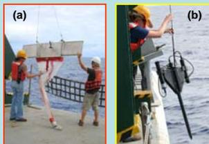
**Figure 3.** Research scientists deploying (a) Manta Trawl and (b) HYPERPRO Radiometer.
