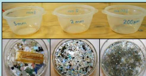
**Figure 4.** Size-fractionated plastic pieces collected from the Manta Trawl.
