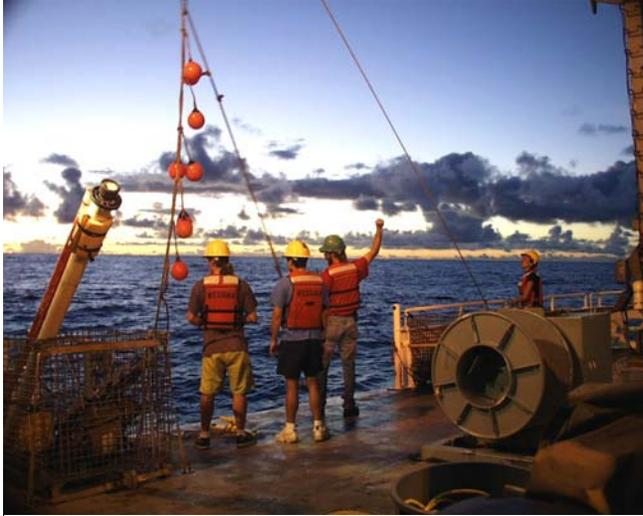
Deployment of the spar buoy off the stern of the R/V Ka'imikai-O-Kanaloa. Image courtesy of HOT/SOEST
